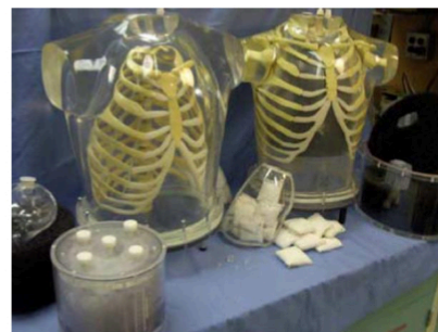
Anthropomorphic phantom modified for mechanical breathing
